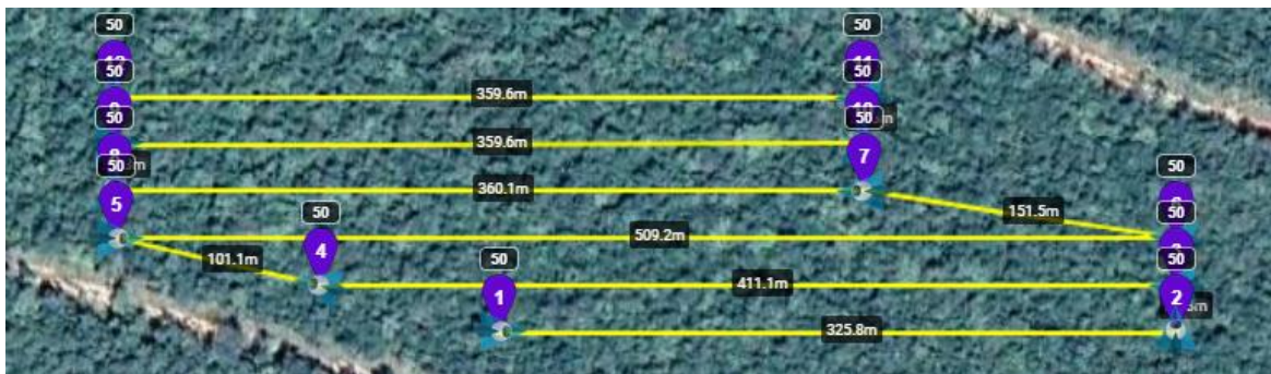
Figure 3. Example of the planned flight path for the RGB drone (yellow line) in a 5-ha sampling site of late regenerating forest as seen in the Litchi Mission Hub. Yellow arrows represent the flight route and the direction in which the drone will fly. The blue balloons represent the boundaries of the sampling site.
