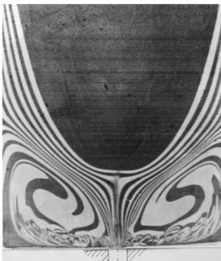
Fig.4 Visualisation of the close-to-critical flow of a LDPE melt Type I at 150°C 3) . The dye pattern in the sliced solidified strand around the center line converges towards the indicated capillary entry below. The circular vortex is a passive closed flow system.
