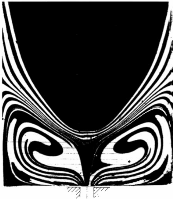
Fig.3 Flow visualization on a slice cut from the middle plane of the frozen LDPE slab after a stopped capillary rheometer experiment 5) .
