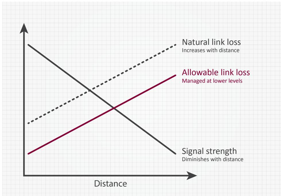
When designing a wireless system it's important to note that all transmissions disperse over distance and that other environmental factors can also affect the strength of the received signal. Link loss increases with range.
